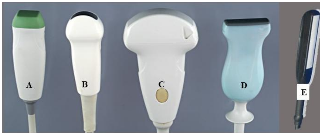
A-Phased array, B-Microconvex, C-Large convex array, D-Linear array, E- Linear array – Rectal
