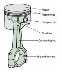
It is a cylindrical part and its closed at the top and opened at the bottom. The piston is made crown on top side to deflect the charge. Three grooves are made on the top side to deflect the charge.Three grooves are made on the circumference of piston to carry the piston rings. Generally it is made with cast iron, cast steel, aluminium alloy and chrome nickel alloy.They are produced by casting or forging.
