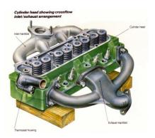
Cylinder head is also a single casting bolted to the top of cylinder block. It consists of combustion chamber, spark plug or injector and valves. Passages or jackets are provided for the circulation of cooling water. It is usually made with grey cast iron or aluminium alloys. A gasket is placed in between the cylinder head and cylinder block to prevent leakages caused by compression.
