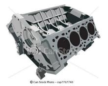
Cylinder block forms the main body of an engine. It contains cylinder to accommodate a piston. It houses crank, camshaft and other engine parts. It is provided with openings for valves and water jackets. Around the cylinders, there are passages for the circulation of cooling water. Generally it is made of a single casting and materials used are grey cast iron or aluminum and its alloys.
