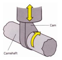
Camshaft is used to operate the valves of the four stroke engine. It is connected to the crank shaft through timing gears or by timing chain.
